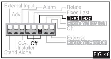
The First On / Last Off or First On / First Off DIP switch selects whether the first boiler is the first to stage on and the last to stage off or the first to stage on and the first to stage off. This DIP switch is only active when the Rotate / Off DIP switch is set to Rotate and the Fixed Lead / Off DIP switch is set to Fixed Lead (FIG. 49).
